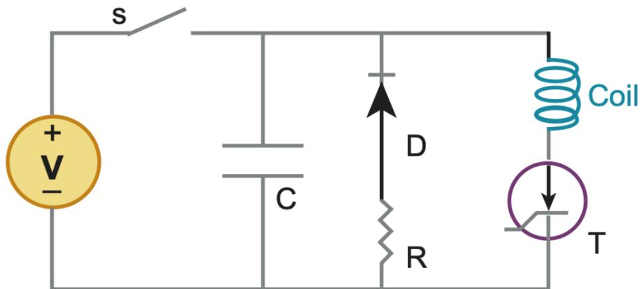
(*V* voltage source, *S* switch, *C* capacitor, *D* diode, *R* resistor, *T* thyristor )
